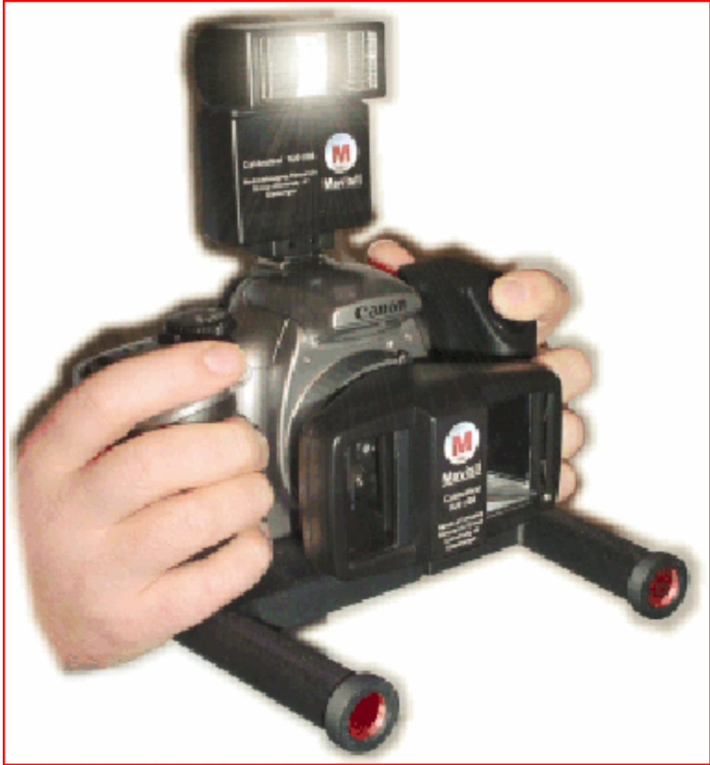
volume measurement: passive vision by dual lens stereovision (MAVIS II)
