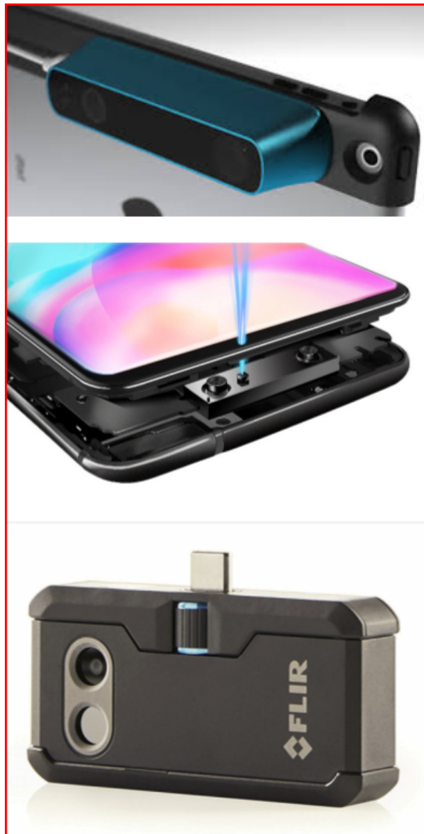
Structure Sensor by Occipital mounted on a tablet (top) Vivo's TOF 3D sensor for smartphone (center) Flir One PRO LT thermal camera for iPhone and iPad (bottom)
